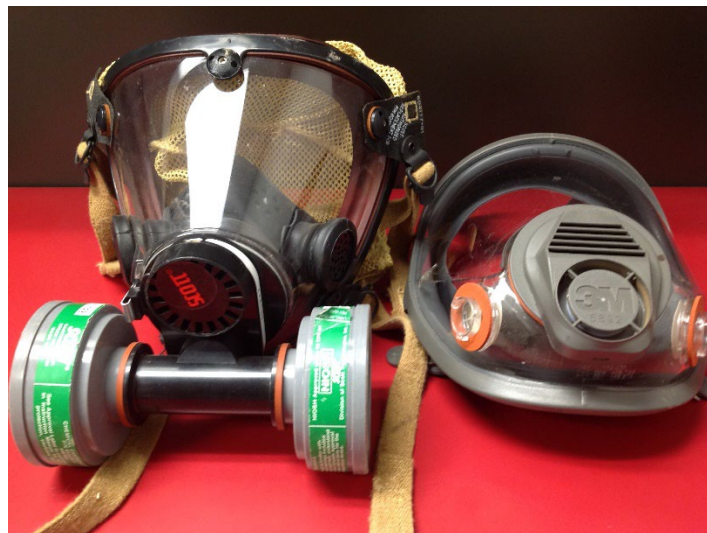
Figure 3: Full-face respirators. The respirator on the left has cartridges installed; the one on the right does not.
